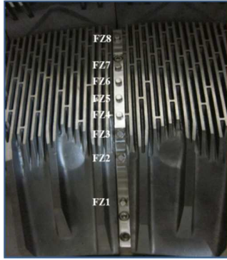
Fig. 7: Sensor array with eight temperature sensors mounted between two refining segments in the flat zone of a CD-refiner.
